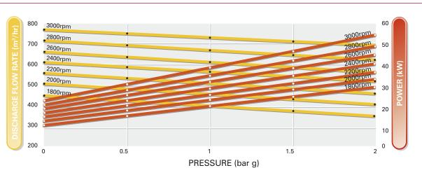
Discharged flow measured in accordance with BS1042/ISO 5167-1/BS ISO TR 15377 and referred to standard ambient conditions (1013 mbar, 20°C)
