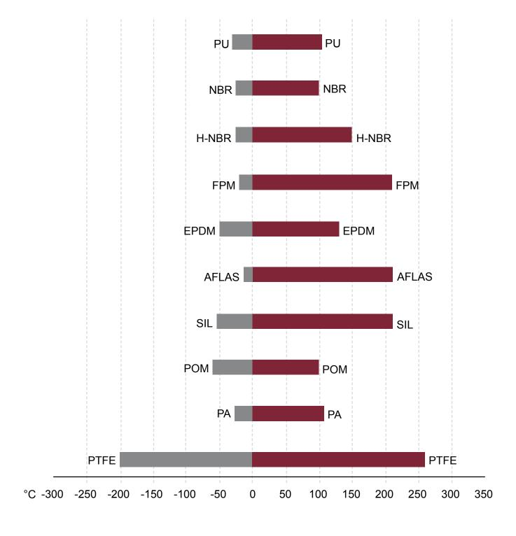
The chart above gives a rough overlook over the application temperature of the most important seal materials. When using a material in contact with a chemically aggressive fluid, these temperature limits can get dramatically reduced.
